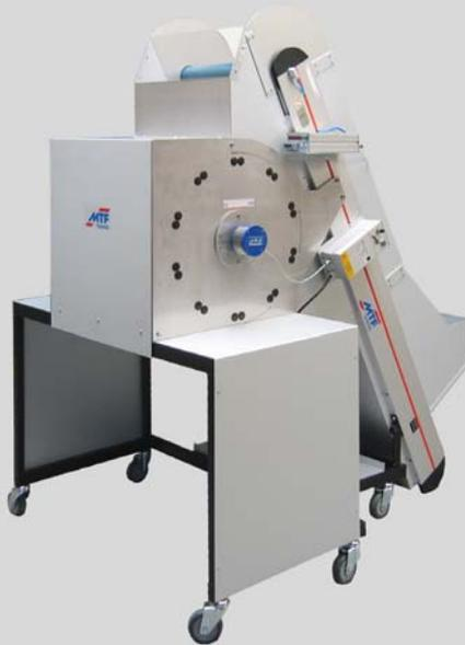
Magnetic Separation Drum with Multi-Tech Feeding Conveyor.
