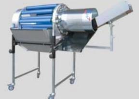
Roller Separation Drum with Perforated Drum Inlet Ring
