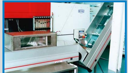
A closed system: The transfer from the injection moulding machine to the MTF conveyor system.
