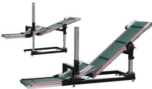
Conveyor Combination with Height Adjustment
