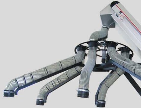
Special System for Automated Conveyance and Distribution of Bottle Caps into Multiple Bulk Containers.
