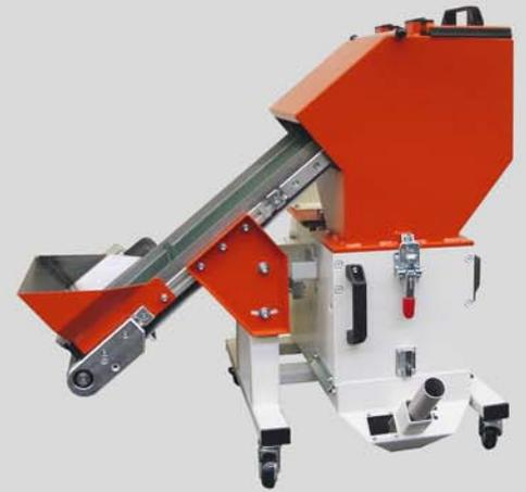
Here are some I-Tech examples with granulator (above), as compact testing solution with tunnel detector (right), or as buffer station for small components (below).
