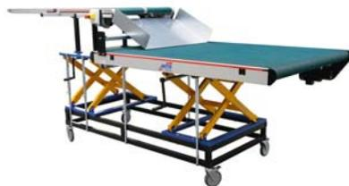
**Height Adjustment by Means of Scissor Lift Tables**
