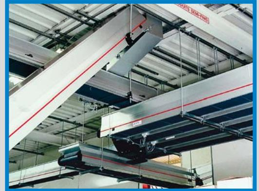
Computer-controlled automation between injection-moulding and printing machines: plastic parts are distributed on further conveyor belts by means of pneumatically adjustable lateral conveyor belts from MTF Technik.
