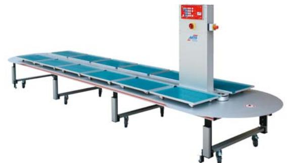
No matter which containers are used - cartons, boxes or bags – the MTF Multi-Line can be adapted easily to the most varied tasks. In particular, the Multi-Line can play to its strengths when the available space is small but relatively long.
