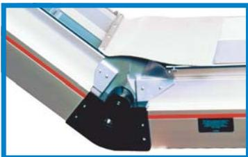
Flexible covering of the adjustable angles, e.g. for clean room applications
