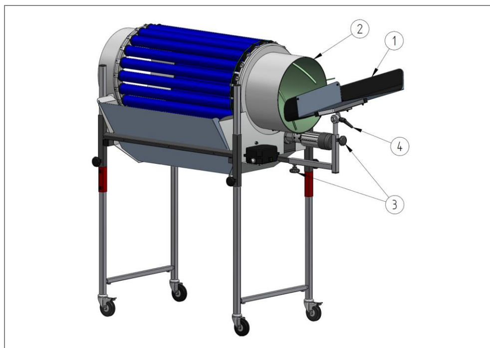
Fig. 12: Inlet chute adjustment options
