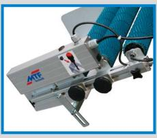
Separation Roller Attachment Type TA Compact control unit with 7 speed steps for the separation rollers. The drive for the separation attachment is integrated in the rollers.
