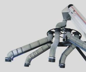
Special System for Automated Conveyance and Distribution of Bottle Caps into Multiple Bulk Containers.
