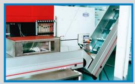
A closed system: The transfer from the injection moulding machine to the MTF conveyor system.
