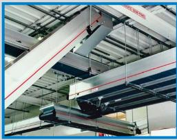
Computer-controlled automation between injection-moulding and printing machines: plastic parts are distributed on further conveyor belts by means of pneumatically adjustable lateral conveyor belts from MTF Technik.
