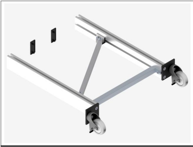
Fig. 27: Assembly of the support – AM 140 (typical)
