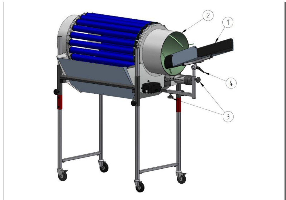
Fig. 12: Inlet chute adjustment options
